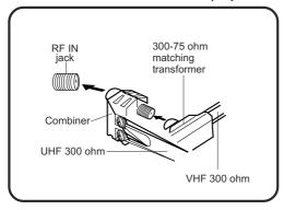
Connect the UHF 300 ohm twin-lead wire to the combiner (not supplied). Connect the VHF 300 ohm twin-lead wire to the 300-75 ohm matching transformer. Attach the transformer to the combiner, then attach the combiner to the RF IN jack.
